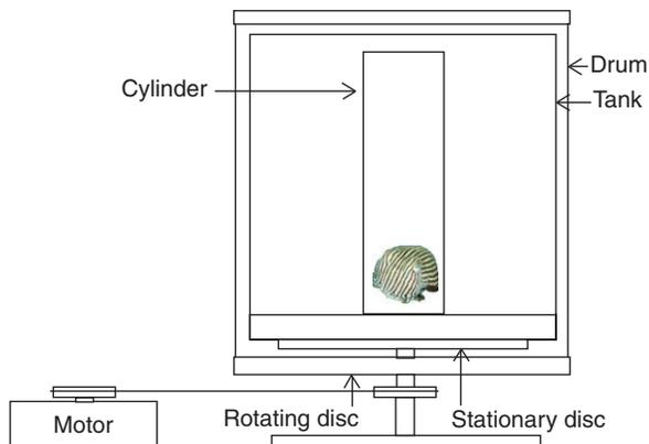
Fig. 4. Schematic diagram of the apparatus used to elicit OKRs in *S. lineolata*. Each specimen was placed into a cylinder inside the tank to prevent them from burying into the substrate.
